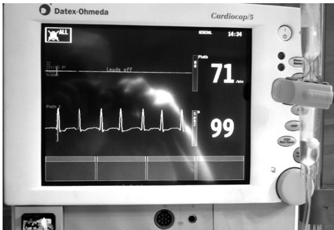
An oxygen saturation probe attached to a drip chamber produced what looked like an ECG and reassuringly normal oxygen saturations
