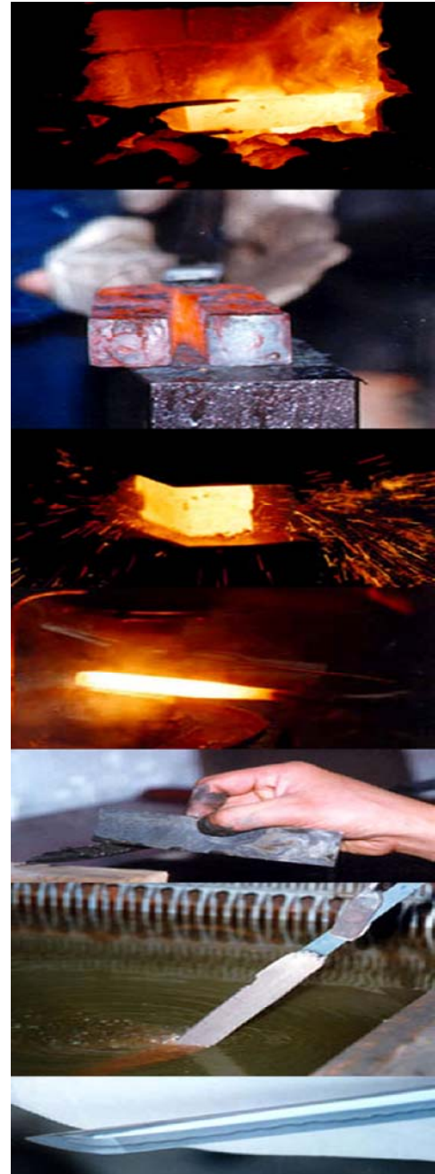
Figure 1 - Process in creating a Japanese Sword, from top to bottom: The steel is heated prior to the forging process in a charcoal fire; After hammering the steel out, it is cut in half and folded; The folded steel is then hammer welded together, as the forging process continues; The smith then continues to shape the blade, first with a power hammer and then with a hand held hammer; After forging, the blade is shaped by hand, and then coated with clay, prior to the hardening process; After the claying of the blade, it is heated to critical (about 1450°F) and then quenched in water, creating the martensite edge and pearlite body of the sword; The blade is then final shaped and polished. This sharpens the blade and reveals the hamon that is created by the hardening process. Figures courtesy Bugei Trading Company.
